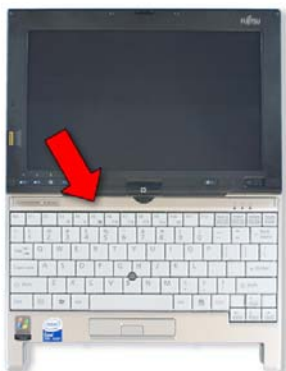
59. Press the keyboard upper trim into place.
