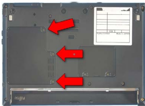
65. Replace the Drive cover and secure it with 3 screws.
