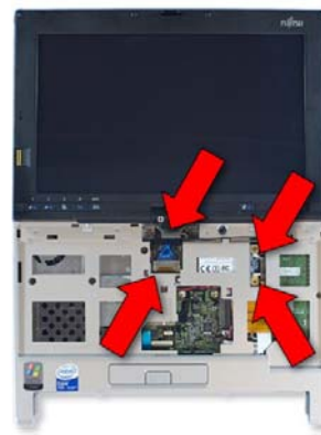
14. Disconnect 2 Display cables from the system board and the 2 antenna cables from the WLAN Card.
