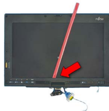
20. Gently slide the pry tool between the screen and the front cover to release the double sided tape located there.
