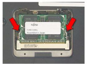
3. Press out on the locking clips to release the RAM, and lift it out.
