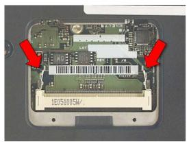
4. Place the new RAM into the slot and press down to lock it.
