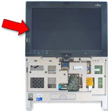
41. Turn the Display back and lay it down.
