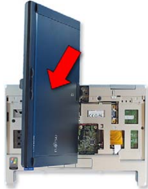
39. Tilt the display up and rotate it ¼ turn.
