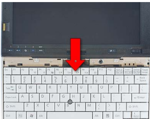
43. Turn the keyboard over and slide it into place
