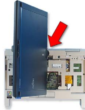
40. Slide the lower hinge cover into place.
