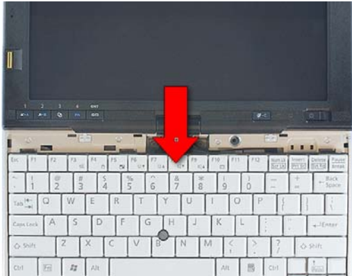
31. Turn the keyboard over and slide it into place
