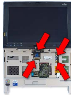
26. Attach the 2 display cables to the system board and the 2 antenna Cables to the WLAN card.
