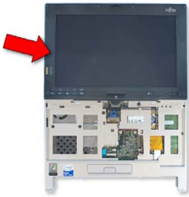
29. Turn the Display back and lay it down.
