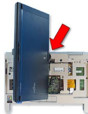
28. Slide the lower hinge cover into place.
