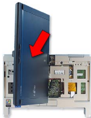
27. Tilt the display up and rotate it ¼ turn.
