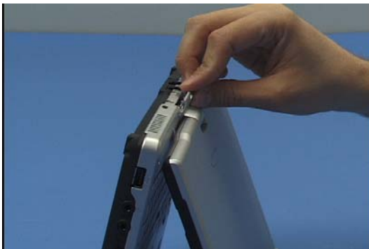
65. Insert the rear hinge cover.
