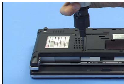
74. Secure the cover with 3 screws.
