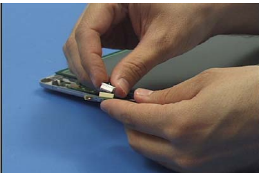
19. Connect the fingerprint scanner PCB cable and place it into the rear cover.
