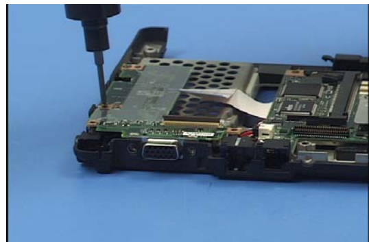
42. Secure the daughterboard with 4 screws.
