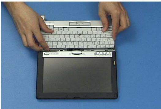
61. Slide the keyboard into place.
