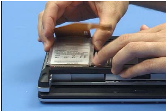
71. Insert the Hard Disk Drive.
