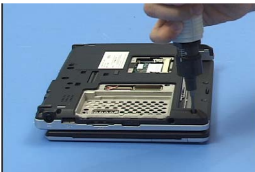
67. Insert 11 lower case screws.
