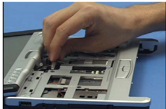
58. Place the metal bracket over the antenna cables.
