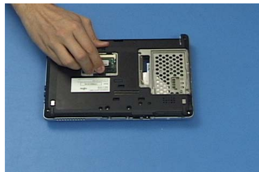
68. Insert the RAM and press it down to lock it.
