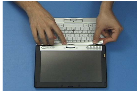
62. Press the keyboard upper cover into place.
