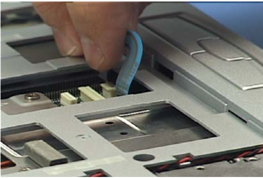
53. Connect the TouchPoint buttons cable.
