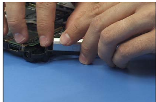
44. Insert the external VGA connector cover into the case.
