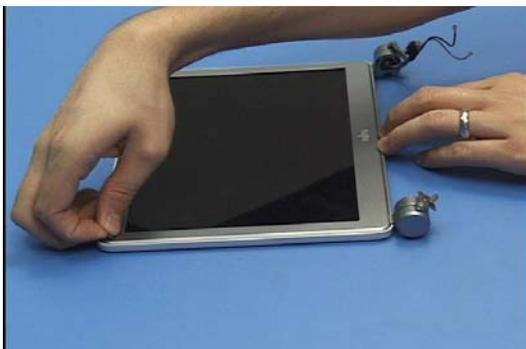
9. Insert 2 screws into the front of the display and cover them with 2 screw covers.
