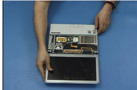
40. Open the display and lay the unit flat.8
