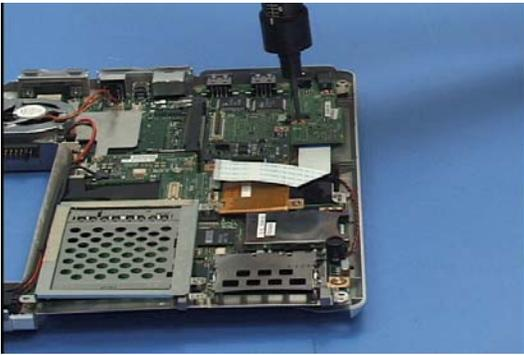
21. Secure the Audio Board with 2 screws.
