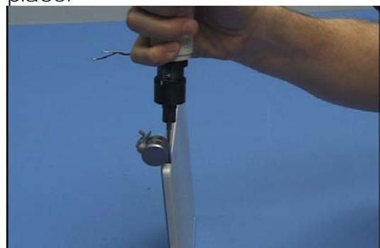
10. Stand the display up on its top and insert 2 screws into the bottom.
