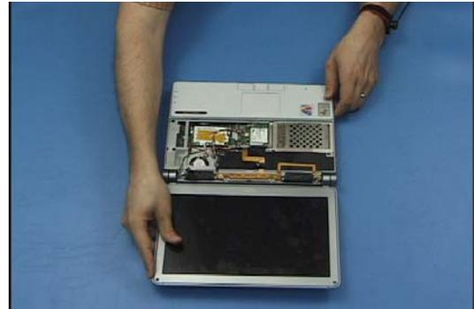
40. Open the display and lay the unit flat.<sup>8</sup>
