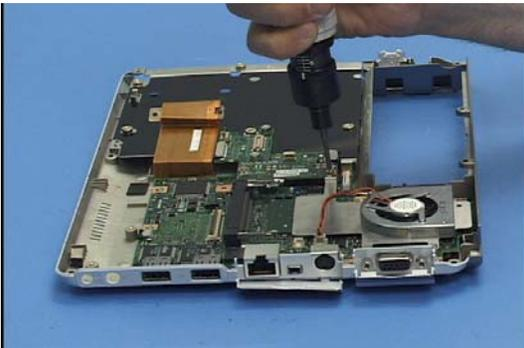
17. Press the Bay Daughterboard onto the system board to connect it and secure it with 2 screws.
