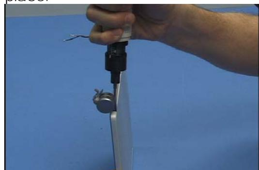
10. Stand the display up on its top and insert 2 screws into the bottom.
