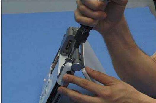
39. Turn the unit up on its front and insert 2 screws into the back of the case.
