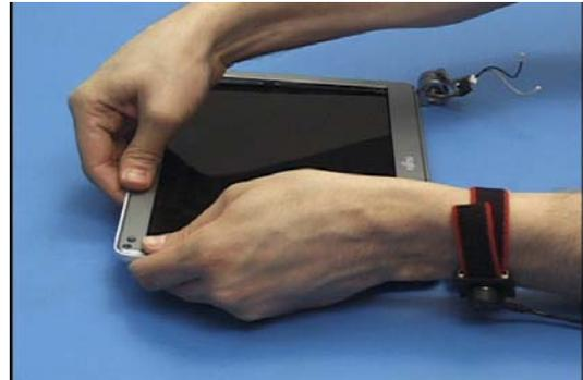
8. Place the front cover onto the display assembly and press firmly around the perimeter to snap it into place.
