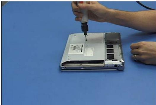
3. Attach the cables to the 2 antennas, place each into the back cover with its metal spacer and secure each with 1 screw.
