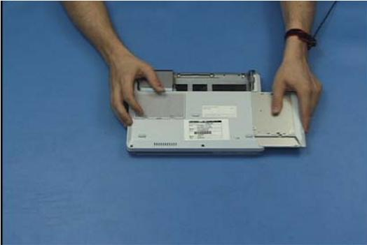
47. Slide the Optical Drive into place.
