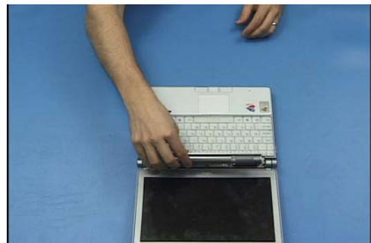
44. Place the speaker/LED cover onto the unit and press it into place.
