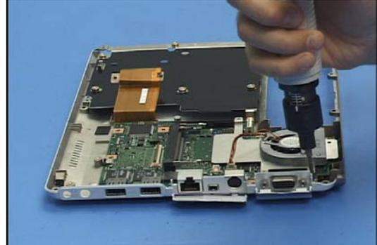
16. Secure the system board with 4 screws.
