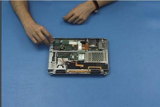
31. Insert the key lock board into the lower case, connect its cable and tape it down.
