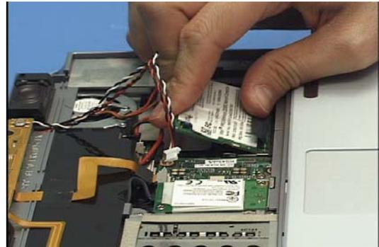
36. Insert the wireless card and apply tape over its contact with the slot.
