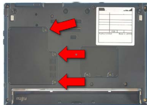
44. Replace the Drive cover and secure it with 3 screws.
