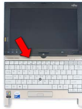
38. Press the keyboard upper trim into place.
