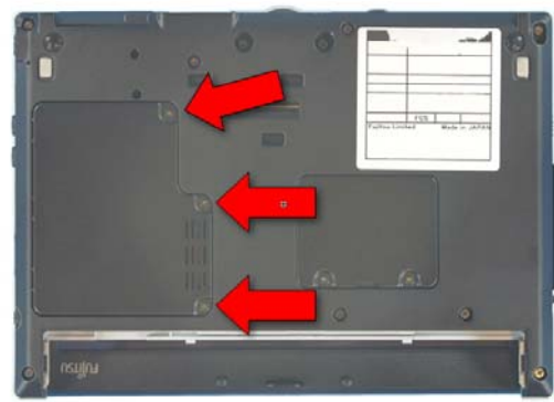
2. Extract these 3 screws from the Hard Disk Drive cover and lift it off.
