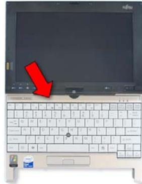
8. Use a plastic pry tool to remove the keyboard upper trim.
