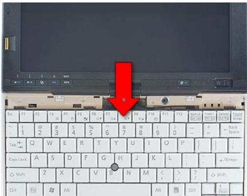
9. Lift the top edge of the keyboard up and turn it over
