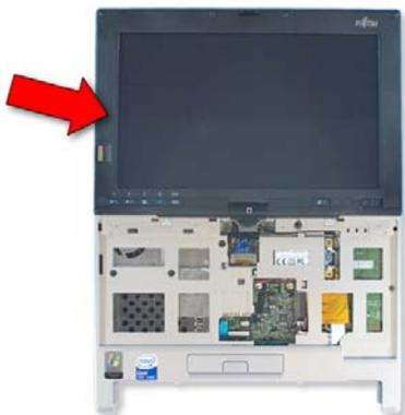
11. Tilt the Display up and rotate it ¼ turn.
