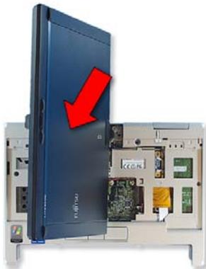
33. Tilt the display up and rotate it ¼ turn.
