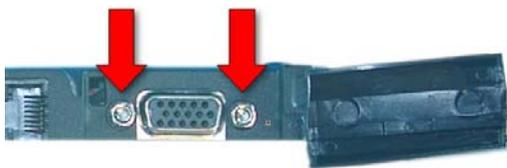
27. Insert 2 hex screws into the external VGA connector.
