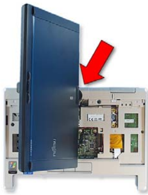
53. Slide the lower hinge cover into place.
