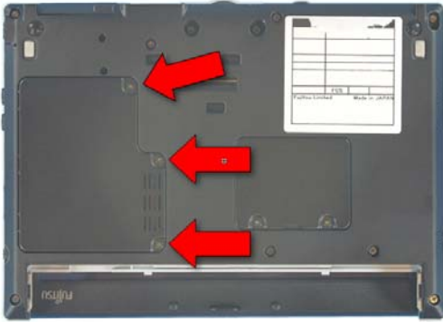
63. Replace the Drive cover and secure it with 3 screws.
