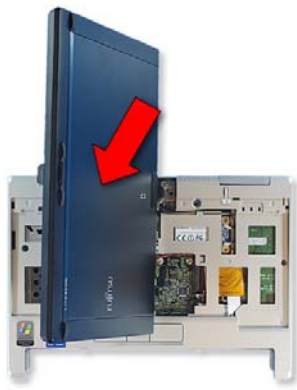
13. Turn the Display back and lay it down.
