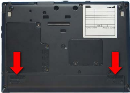
1. Turn the LifeBook over and remove the battery
