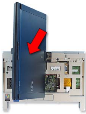
13. Turn the Display back and lay it down.
