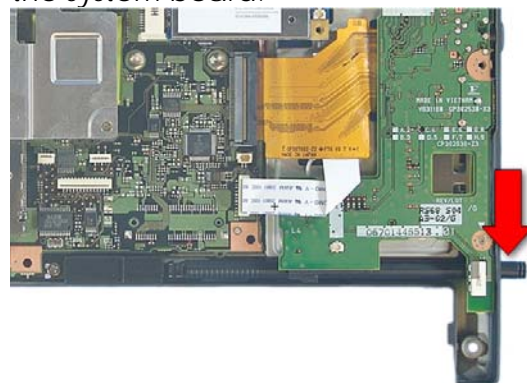
20. Press the stylus to release it and slide it out.
