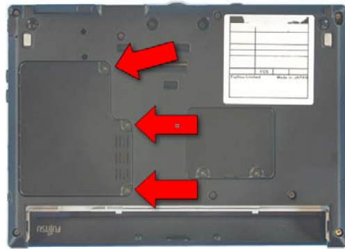
2. Extract these 3 screws from the Hard Disk Drive cover and lift it off.
