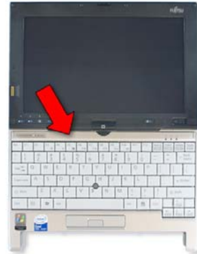
32. Press the keyboard upper trim into place.
